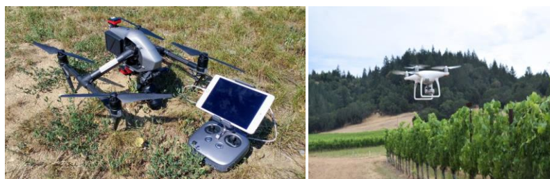
Figure 1. (a) UAV equipped with multispectral sensor, GPS device and digital camera (Tanda and Chiarabini, 2019) (b) an UAV in precision viticulture
