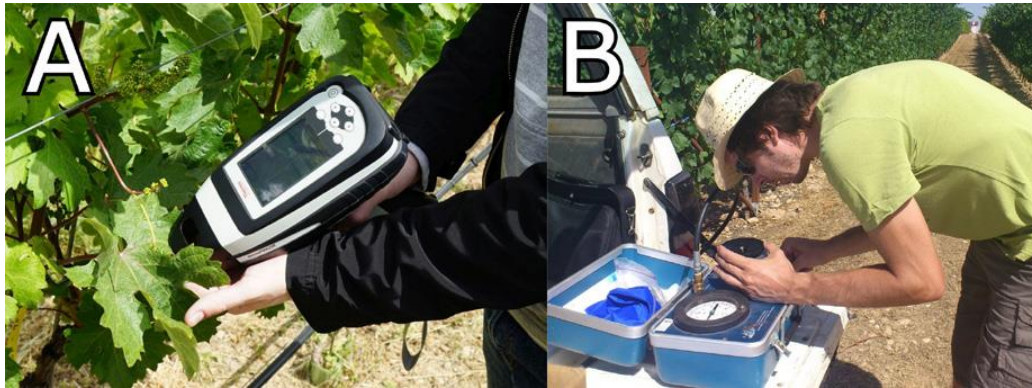
Figure 6. (A) Acquisition of spectral measurements using a portable NIR analyser microPHAZIR™. (B) Measurement of stem water potential (Gutiérrez et al., 2016)
