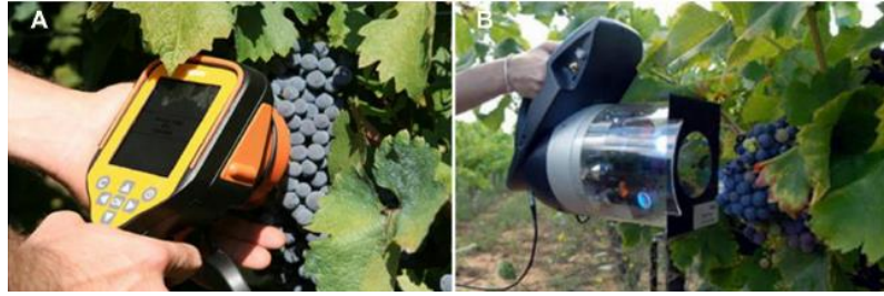
Figure 7. Spectron ( A ) and Multiplex ( B ) hand-device sensors for grape quality proximal monitoring, which allows quality maps to be realized. (Ghozlen et al., 2010).
